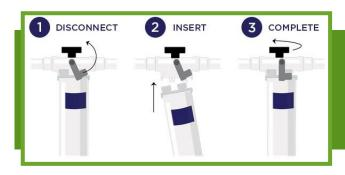
The disposable housing quick connects to the manifold head assembly. The removal of the housing is quick, clean and efficient.
