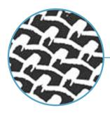
Monofilament Mesh is a woven fabric where each thread is a single filament, boasting excellent strength with no fiber migration. Providing extra strength and abrasion resistance, and offering a broad range of chemical compatibility, Monofilament Mesh bags are available in nylon, polyester and polypropylene.
